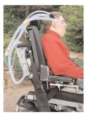
My setup starts with an air tube straw, connected to a 3.5 mm adapter ET, connected to a patient circuit, connected to a bacterial/viral filter and
